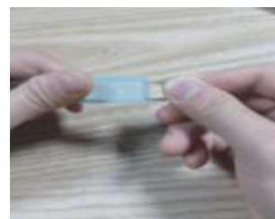
Insert power pin into the other end and connect 4 wires inside.
