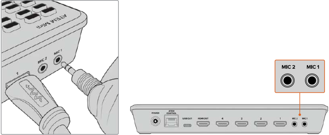
Connect microphones to ATEM Mini's mic inputs
