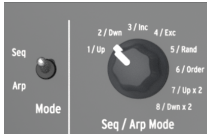
The Mode switch and Seq/Arp Mode knob
